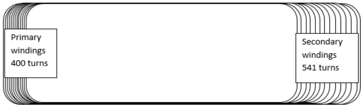
Figure 2: laminated core primary and secondary windings
